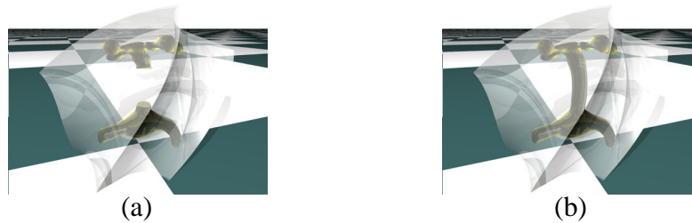
Figure 7.12: PDE-based free-form shape blending and deformation. (a) is two embedded objects to be blended; (b) is the blending result.
