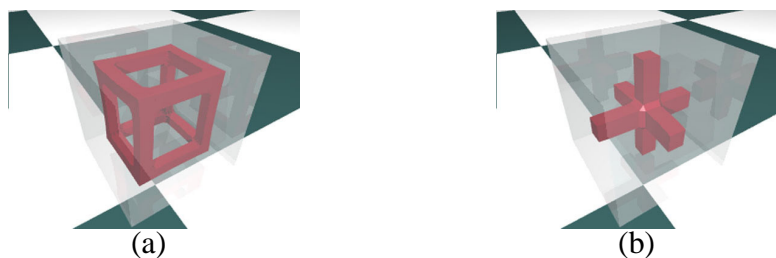
Figure 7.7: Examples using CSG trimming operation in a PDE solid. The trimmed parts are shown in red covered by transparent original solids.
