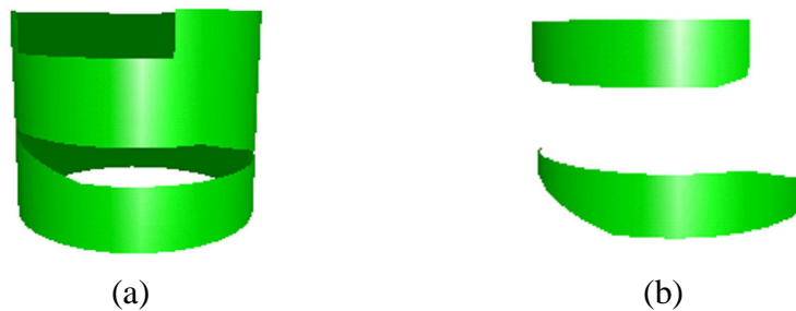
Figure 4.14: Trimming on the selected regions. (a) The surface after the removal of the selected regions; (b) the surface after the removal of all non-selected area.
