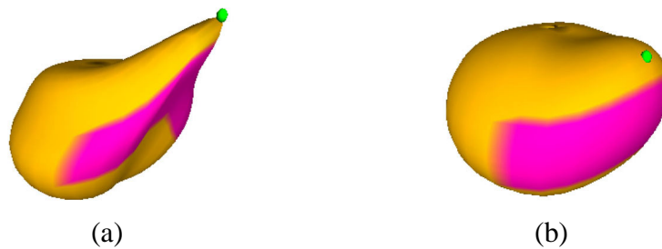
Figure 4.18: The PDE surface sculpting with physical constraints. (a) Directly changing a point of a mass-spring model; (b) point editing in B-spline approximation for the mass-spring model, and the color mapping shows different material properties (refer to Table 9.4).
